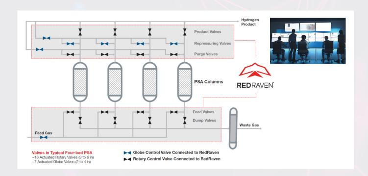
Pressure swing adsorption (PSA) is vulnerable to production constraints when control valves fail or deviate from expected behavior. RedRaven provides insights on equipment health and allows plant operators to proactively identify and address issues before they cause downtime and operational disruptions. Its remote monitoring capabilities coupled with experienced Flowserve support facilitates quick resolution of identified problems.
